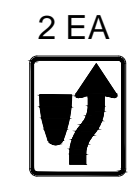
R4-7 (24" x 30") - SIGN, TYPE III B RETROREFLECTIVE WHITE BACKGROUND
