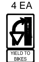
SIGN A (24" x 30") - SIGN, TYPE IIIA RETROREFLECTIVE RED YIELD SYMBOL RETROREFLECTIVE GREEN BIKE LANE SIGN B (24" x 12") - SIGN, TYPE IIIB RETROREFLECTIVE WHITE BACKGROUND
